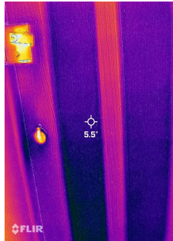
Thermal imaging of a curtain with and without a thermal lining - a difference of 9 degC
